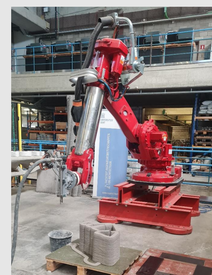
Fig 6: First 3D-printing test
