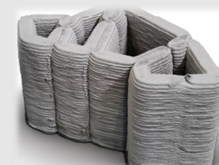
Fig 7: 3D-printed & carbon-cured block
